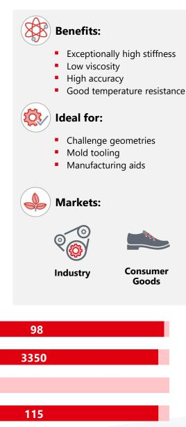
Tensile Stress at Break (MPa)98Young's Modulus (MPa)3350Elongation at Break (%)5HDT at 0.455 MPa (°C)115IZOD Impact (Notched, J/m)24Shore Hardness (3s)88
