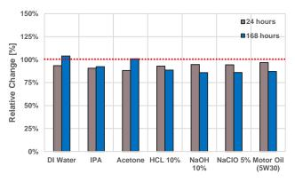
Flexural Strain at Break after Immersion Time
